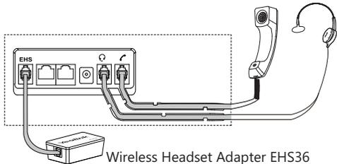
**Note:** The headset or wireless headset adapter EHS36 should be purchased separately. EHS36 is used for connecting the phone and a compatible wireless headset. For more information on how to use the EHS36, refer to Yealink EHS36 User Guide.
