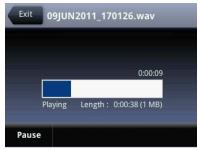
If the handset is off-hook when you play a recording, the audio plays through the handset. If the handset is on-hook when you play a recording, the audio plays through the speaker.
