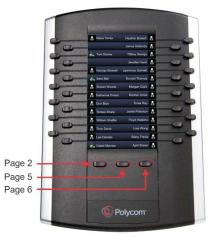
If you have three expansion modules connected to your VVX phone, the pages are ordered non-sequentially. As shown in the next figure, the pages display on the three expansion modules in the following order:
