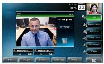
A green bar on the line key indicates the line has an active call, and a flashing red bar indicates the line has one or more held calls.
